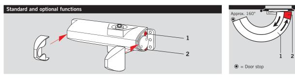
The **closing speed** of the DORMA TS 90 Impulse is adjustable in two independent ranges at the valves indicated. With the DORMA TS 90 Impulse, the **closing force** is permanently set at EN 3.
