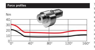
The heart-shaped cam and the linear drive mechanism of the DORMA TS 90 Impulse ensure that the resistance encountered decreases almost instantly with the door opening action – so even children, the elderly and people with disabilities have no problem in opening the door. User-friendly and reliable closing is also ensured by the delayed increase in the actuating torque at the "latching" end of the sweep.
