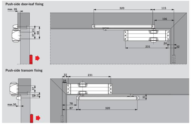
Depending on the structural conditions, the door opening angle is likely to be limited to approx. 95°. It is recommended to install the cushioned limit stay or position a door stop at this point.
