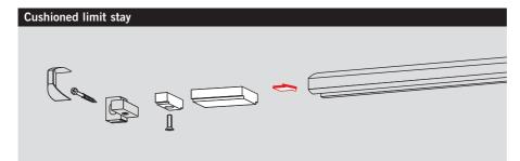
Cushioned limit stay for retrofitting by insertion in the slide channel. Adjustable between 80° and max. 120°.
